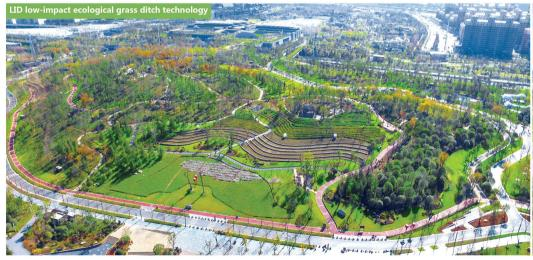
The LID low-impact ecological grass ditch technology is adopted to set up an ecological grass ditch on the hill every five meters, in which soil-retaining plants are planted in the grass ditch to minimize the erosion
